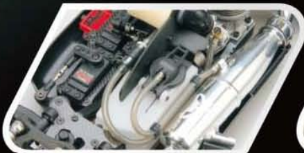
Low Center of Gravity Fuel Tank
