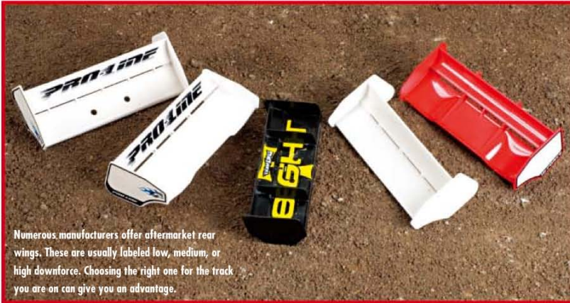
Many kits are designed to allow racers to change the wing angle. A taller angle increases downforce, while a shallower angle (more level) reduces downforce.
