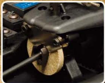
Independently adjustable front and rear disk brakes let you adjust the braking bias to suit your track conditions
