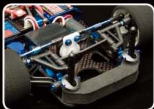
Updated active strut front end features symmetric components with adjustable caster and track width, as well as a new front axle with wheel nut.
