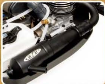
Team Associated 2-chamber muffler and header pipe are designed to provide maximum power to the Pro.28 engine.
