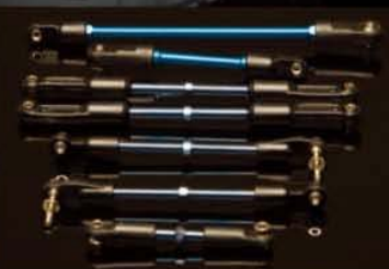
Factory Team blue titanium turnbuckles and aluminum chassis braces come assembled
