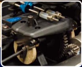
Independently adjustable front and rear disk brakes lets you adjust the braking bias to suit your track conditions
