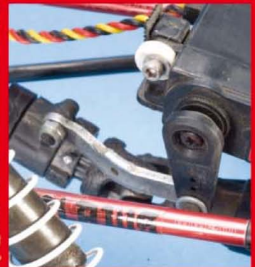
Free wheel dig allows the rear tires to follow the front without pushing. Pushing may cause the rear to slide or raise the CG, which may cause a rollover.
