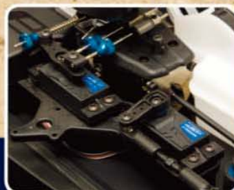
Team Associated's S2008 metal gear high-torque steering servo is tough and comes standard in the SC8
