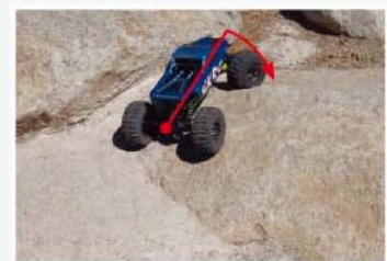
Here you can see how the rear stays relatively in place while the front pulls the truck in a tight arc. This redirection would take many reverses without the use of a locked dig, especially when courses are set up tightly.
