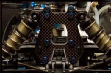
Factory Team carbon fiber shock towers for light weight strength and durability
