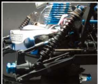
Hard-coated, threaded shocks with rubber boots keeps the suspension smooth
