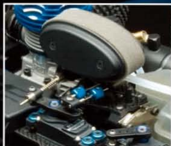
Low-profile elliptical high-flow, two-stage air filter and FFC brake system
