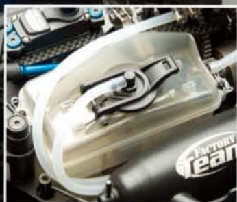
Anti-foaming fuel tank is quickly and easily removed with two clips
