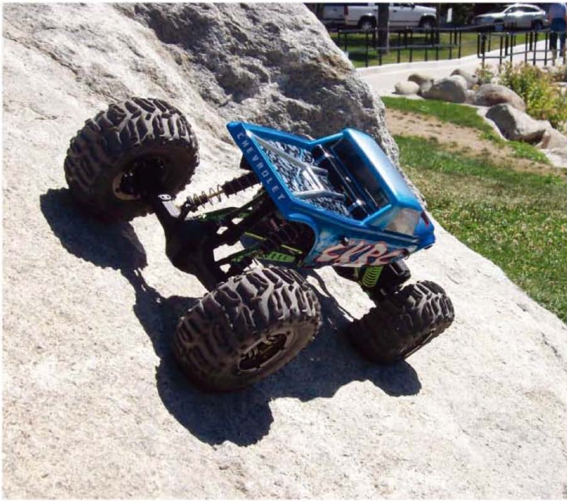
Free wheel dig allows the rear tires to follow the front without pushing. Pushing may cause the rear to slide or raise the CG, which may cause a rollover.
