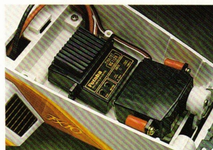
The MC112B is ideal for offroad cars like our FX10. It features MOS/FET design with reverse and installs conveniently in place of the throttle servo.
